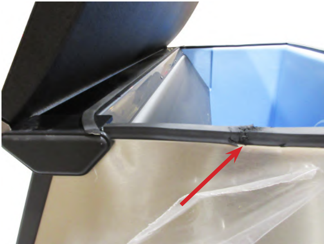
Minor gasket damage
