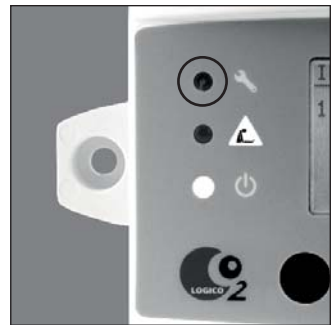
System fault indicator
