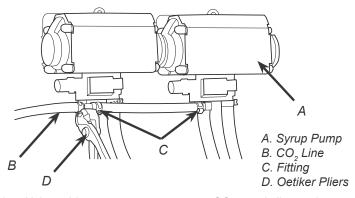
Using tubing cutters, cut any pump CO<sub>2</sub> supply line and install tee fitting, then route appropriate tubing from the CO<sub>2</sub> supply to the tee fitting at syrup pumps.
