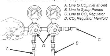
Using a wrench, loosen lock nut on the regulator adjustment screw of the high pressure CO<sub>2</sub> regulator connected to the source, then using a screwdriver back out lock nut screw all the way.
