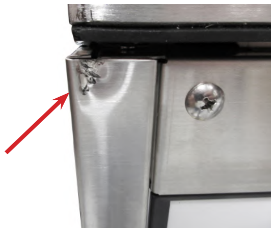
Minor door frame damage close-up
