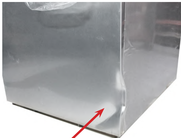
Dent damage close-up
