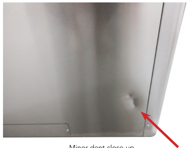
Minor dent close-up
