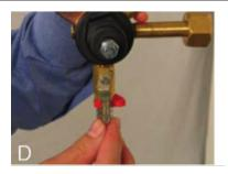
Open the shutoff valve on the regulator to allow gas to flow from the regulator to the keg coupler. You will now hear the keg pressurizing. The output pressure needle will drop momentarily and the return to your set pressure once this is complete.
