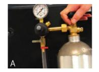
With the shutoff valve on the regulator closed, open the valve on the gas cylinder completely. The handle on the shutoff should be perpendicular to the tubing.
