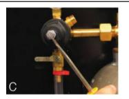
Slowly turn the regulator adjustment screw or knob clockwise until the desired pressure is shown on the on the output pressure gauge. Turning clockwise will increase the output pressure and you will feel greater resistance as psi setting goes up. Tighten the adjustment screw or snap the cap back down to "lock in" your pressure setting.
