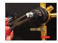
With your fingers or a pair of pliers, loosen the adjustment nut, allowing the screw to be turned. Turn the screw counterclockwise until it can no longer be turned.
