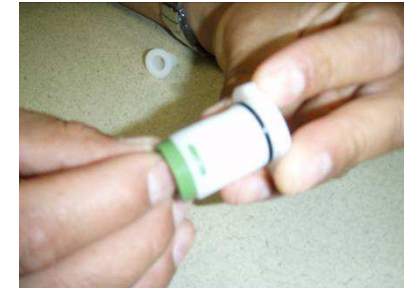
Valve should lock in place with valve housing
