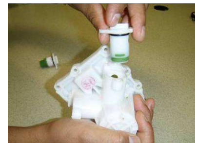
Insert Outlet valve assembly in outlet ports of pump
