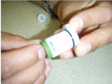
Outlet valve assembly
