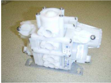
Flush 4:1 Brix Pump according to sanitization procedure
