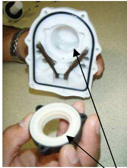
Insert new plunger seal in to syrup housings
