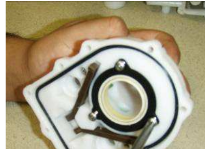
Secure plunger seal in place by inserting screws which were removed and hand tightening (6 – 8 in/lbs torque)
