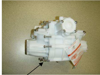
Remove outer body screws (9 per side)
