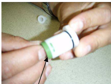
Apply a small amount of grease to the inside of the outlet valve
