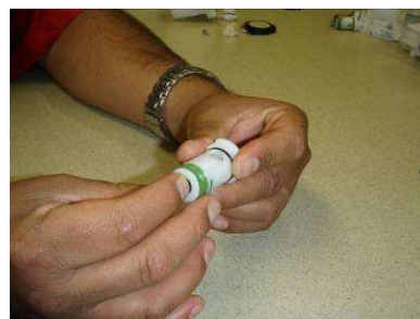
Carefully Insert outlet valve support
