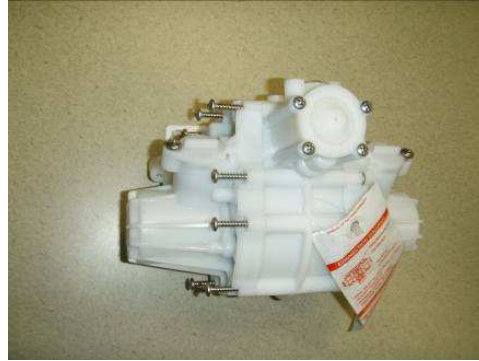
Insert all 18 screws and hand tighten (12 – 15 in/lbs torque
