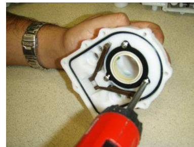
Remove 3 screws from plunger seal (Both sides)
