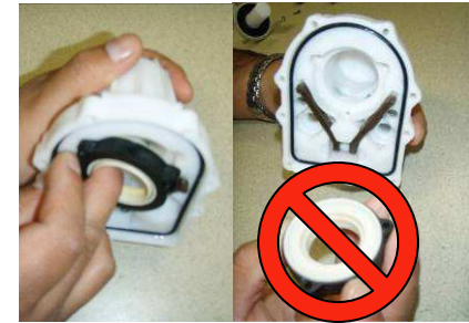
Remove plunger seal and discard it
