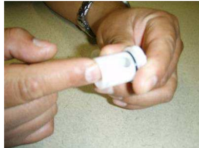
Apply a small amount of grease to the inside of the outlet valve assembly
