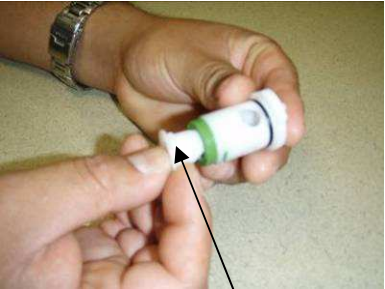
Remove outlet valve support
