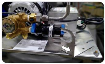
clockwise to reduce the by-pass pressure setting.
