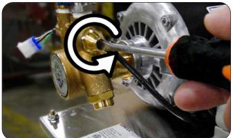
3. Rotate pump head counter-clockwise to access bypass screw.
