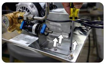
4. Visually identify the slotted-screw head for the bypass adjustment.
