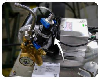
6. Once complete, rotate pump head clockwise back down to original position, rotate lock-bracket back over into place and tighten the 3 deck screws.
