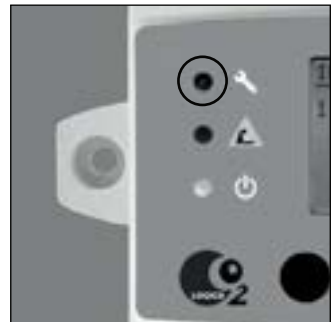
System fault indicator
