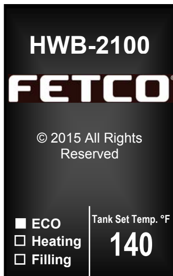
ECO mode icon displayed Unit is in ECO mode after being idle for more than four hours
