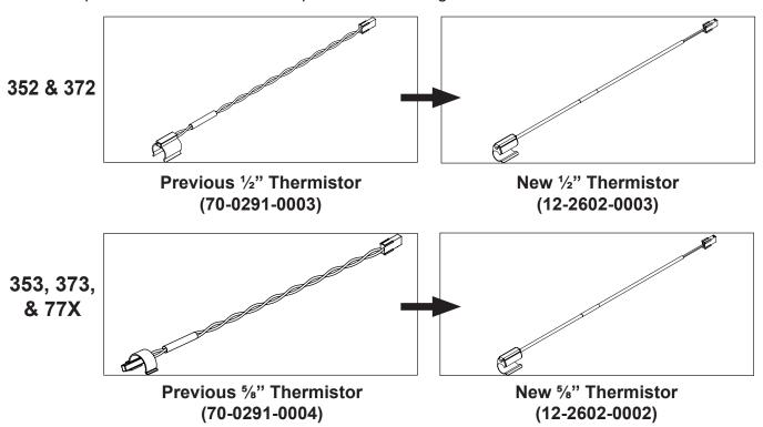
The new thermistor is a drop-in replacement and was implemented into dispensers in the San Antonio facility in May 15, 2020 starting with serial number 20050230.
