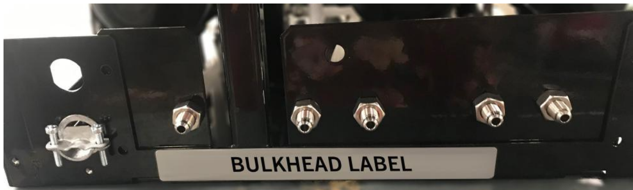
Figure 4.3 Bulkhead Fittings Label Location
