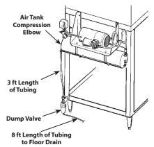
Mounting the Dump Valve onto the Multiplex Refrigeration Unit
