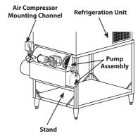
Mounting the Air Compressor onto a Multiplex Support Stand
