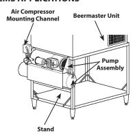
Mounting the Air Compressor onto the Beermaster™ Unit
