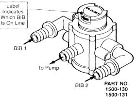
Recommended installation for C02 Pumps or Electric Pumps
