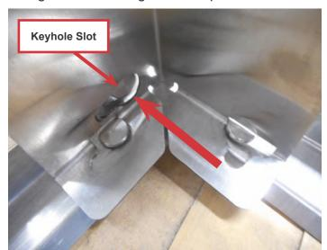
3. With the leg against the inside edge of the top rim, use a rubber hammer or mallet to engage all three (3) rim buttons in the elongated slots.
